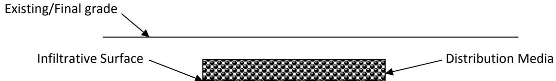
However in a few instances, such as in the definition of “mound”, and within section 43.11(C), which refers to “mounded sand filters”, these items reference two separate interfaces. The top surface of the treatment media (C33 sand) is one “infiltrative surface” and the surface of the native soil below the treatment media is the other “infiltrative surface”. Refer to the mound system drawing below:
